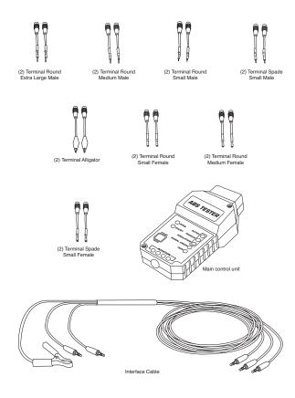
The ABS Sensor Pinpoint Tester and Flex Probe adapters quickly and easily isolate the sensor from the vehicle harness and control module. The tester checks both active and passive sensors for proper voltage, frequency output and reluctor wheel (tone ring) integrity. The tester will also check the passive sensor for opens and shorts.
