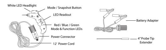
White LED Head lamp—Turns on automatically at power up.
