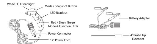
White LED Head lamp—Turns on automatically at power up.
