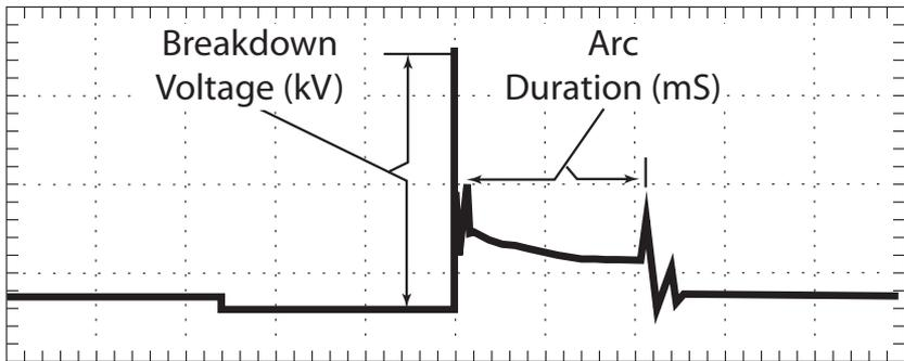
Oscilloscope Secondary Waveform Characteristics
