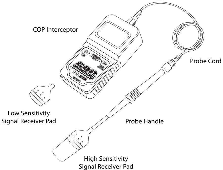
**COP Interceptor**— Used along with the supplied accessories listed below, the COP Interceptor measures a coil on plug's secondary circuit's breakdown voltage (kV) and arc/burn duration (mS) in real time.
