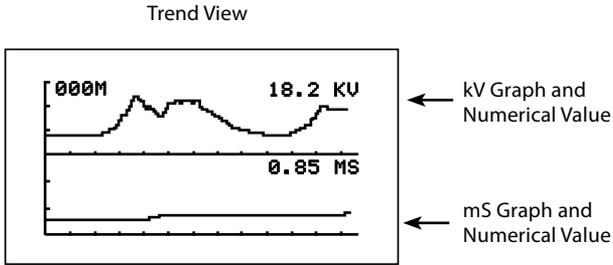
Tapping the left function key pauses the screen. A blinking letter "P" is displayed at the top of the screen while in pause mode. To resume trending, press the left function key.
