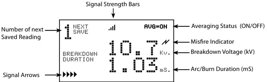
Tapping the left function key saves the reading for later viewing in Balance View. You can save up to eight readings. Any additional readings after eight will overwrite the previous information beginning with saved number one. The number of the next saved reading is shown in the upper left corner of the screen.
