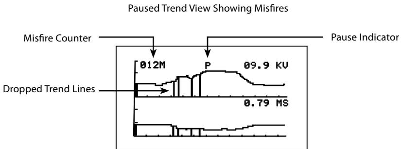
*Note: It is possible to see occasional misfires even if a coil is firing normally. If this happens after running Auto-Set, repeat using a different signal pad receiver or adjust the sensitivity (misfire trigger) in the setup menu.*
